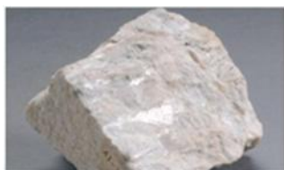
plagioclase feldspar - NaAlSi_3O_8 sodium (chemical symbol Na) and/or CaAlSi_2O_8 calcium (chemical symbol Ca) instead of potassium
