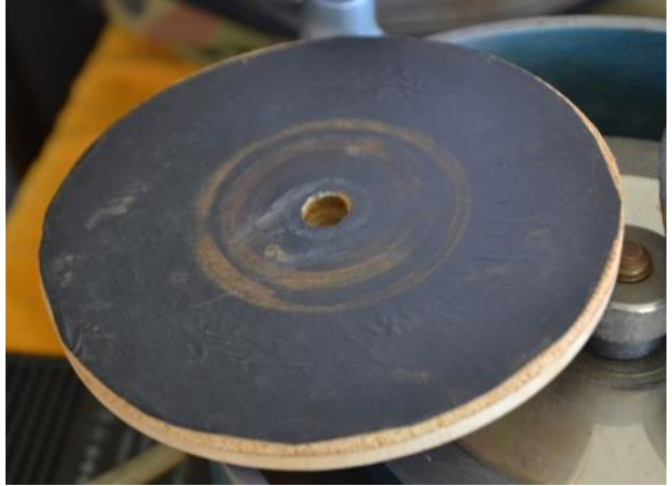
Wet & Dry Emery paper on wood and rubber foam
