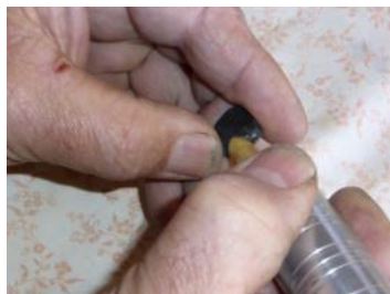
Polishing a sapphire bomb with wooden dowel
