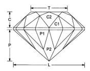
Angles for R.I. = 1.540 57 + 16 girdles = 73 facets 8-fold, mirror-image symmetry 96 index L/W = 1.000 T/W = 0.516 U/W = 0.516 P/W = 0.435 C/W = 0.218 Vol./W³ = 0.241
